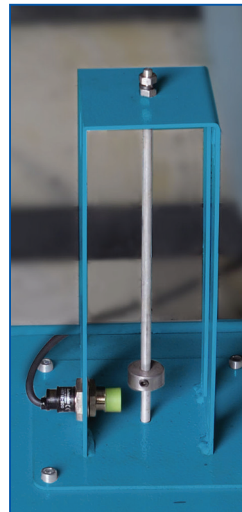
Coolant Feed Controller – Detects the flow of coolant feeding while the saw is in operation.
