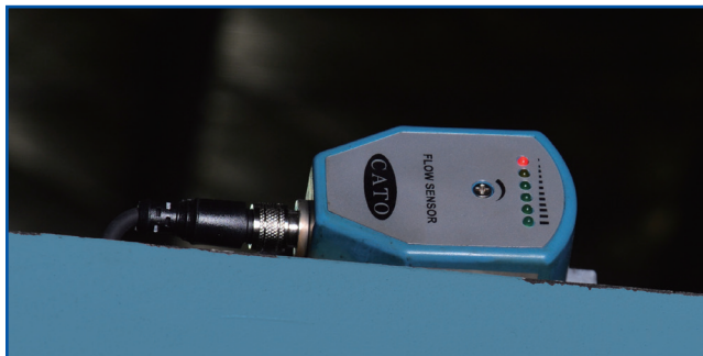
Coolant Feed Controller – Detects the flow of coolant feeding while the saw is in operation.
