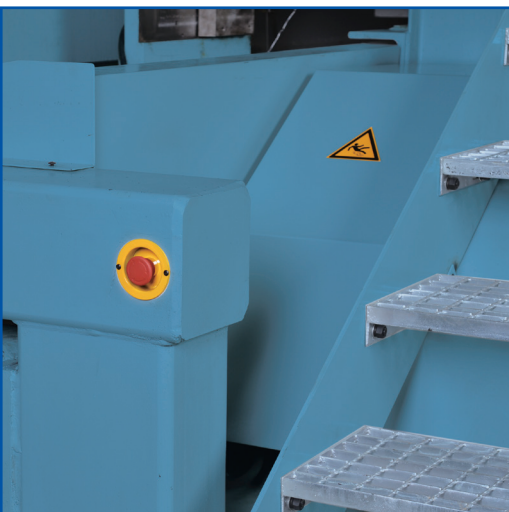
Emergency Shut-Off Buttons – There are 3 emergency shut-off buttons to stop the saw that can be controlled even if the operator is not near the control panel.
